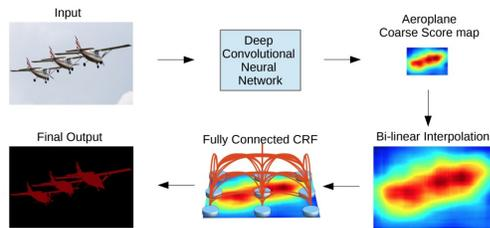
Fig. 10. A CNN+CRF model. From [36].
