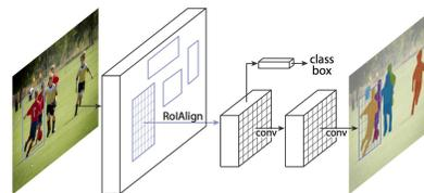
Fig. 18. Mask R-CNN architecture. From [62].
