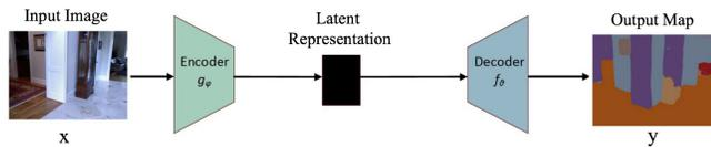
Fig. 5. Architecture of a simple encoder-decoder model.
